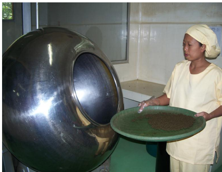
Figure 38: A large jamu industry employee puts a tray of round herbal pills into a machine that helps condense and shine the product. PT Jamu Simona.
